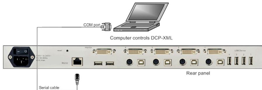
Use the serial cable to connect the COM port of the Windows computer with the serial port of your SPLITMUX-DVI-4.
